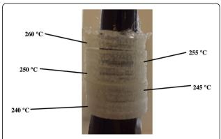
**Fig. 5** 3D printing temperature effects on the transparency. With increasing printing nozzle temperature the transparency increases
