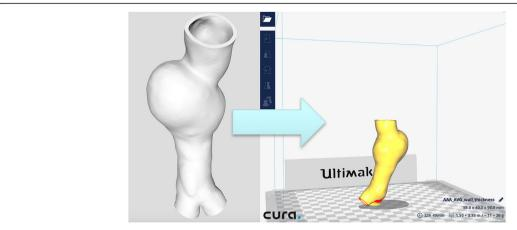
Fig. 1 Picture of the 3D reconstruction from the patient's AAA geometry. The picture was obtained from CT scan data, which was transferred to the software Cura (version 2.5, Ultimaker, Geldermalsen, Netherlands) for layer slicing and setting the 3D printing parameters
