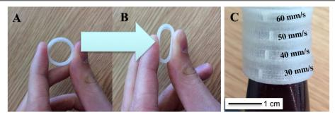
**Fig. 3** 3D printed rings with 2 mm wall thickness for the application of AAA modelling. **a** and **b** The 3D printed rings are flexible. **c** Rings printed with 30, 40, 50 and 60 mm/s printing speeds (see Additional file 1: Table S7 in the Appendix for the rest of the printing parameters) had fair transparency and a noticeable join line that was constant throughout all prints
