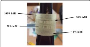
**Fig. 4** The infill density changes the sample transparency. The 100% infill density displays better transparency than the 0% infill density. The 20 and 50% infill densities have partial layer fill, clouding the transparency. With 100% infill the sample is has no air gaps; thus, no clouding of optical properties appears
