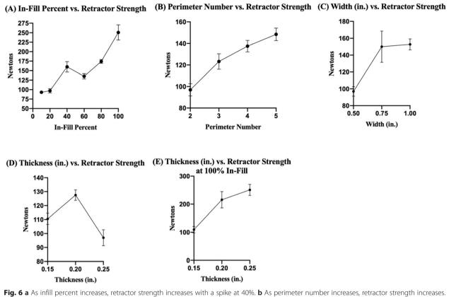
Fig. 6 a As infill percent increases, retractor strength increases with a spike at 40%. b As perimeter number increases, retractor strength increases. c As retractor width increases, retractor strength increases up to 0.75 in. d Retractor thickness is most optimal at 0.2 in. at 20% infill. e Increasing retractor thickness increases retractor strength at 100% infill
