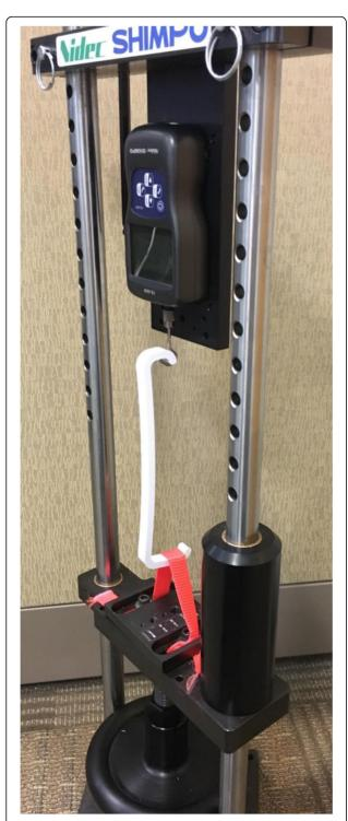
**Fig. 2** Nidec-Shimpo FGS-1000H hand wheel test stand and FG-3009 force gauge with oriented retractor
