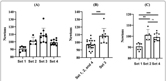
Fig. 5 a Interspool and inter manufacturer variability affects control retractor strength. b Intermanufacturer variability affects control retractor strength. c Interspool variability affects control retractor strength
