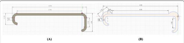
Fig. 1 a Standard retractor design and b reinforced retractor design in inches. c The Army-Navy retractor is oriented on the print bed horizontally such that no support material is needed
