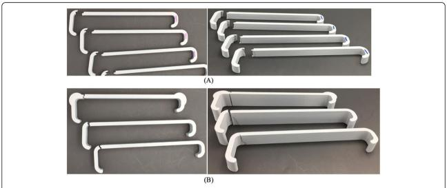
Fig. 4 a Broken standard retractors and b broken retractors with (top to bottom): 1 in. width with reinforced joints, 1 in. width, and 0.75 in. width
