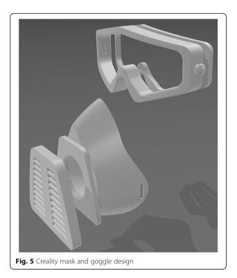
layers of folded fabric or filters (Fig. 5). The Creality goggles require separately sourcing transparent plastic inserts, which may be obtained from repurposed household items. As with all masks, judicious testing for seal adequacy and experimentation with sizing and materials are required for implementation.
