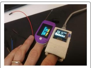
Fig. 1 Comparison between a home-made pulse oximeter against a certified one
